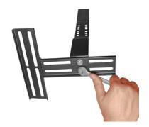
1) Attach one pair of brackets with screws, washers and nuts provided. Leave them loose enough to allow outer bracket to slide (these nuts need to be tightened on step 3). Repeat with the second pair of brackets with the outer bracket facing the opposite side. Base unit needs to be on a flat surface with the top side facing down before continuing with step 2.
