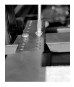
2) Join the bracket to the bed frame as you need it. Select a hole that will leave a space between 1.5" (38 mm) and 2" (51 mm) between the edge of the base and headboard brackets. Continue with next steps of base assembly before proceeding to next step of attaching headboard legs.
